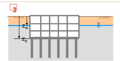
This case is interesting because of the computation of the tensile load  $F_t$  on the anchors/anchor piles
